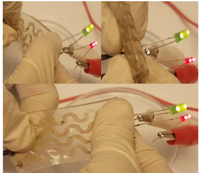
Figure 4. The performance of the fabricated multiple tracks when it is twisted, bent and stretched.
