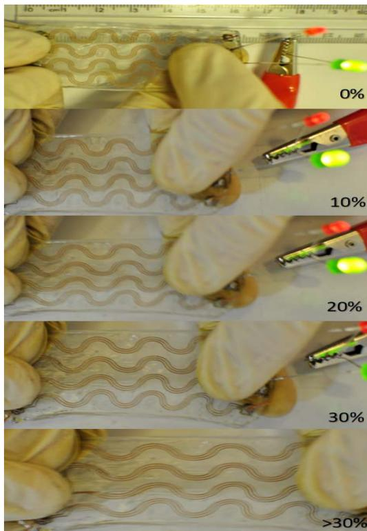
Figure 5. images of LEDs with multiple track interconnects with elongations ranging from zero to more than 30%. The LEDs were ON during the test.
