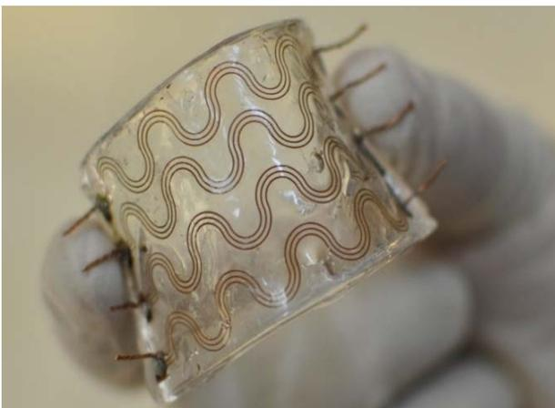
Figure 1. camera image of fabricated stretchable interconnects. 3 parallel tracks are embedded in PDMS.
