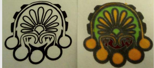
Figure 4. The logo of Amirkabir University of Tehran, fabricated by wax printing procedure and colored by edible color solution.
